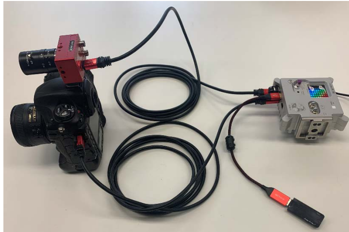
Figure 1: The payload ground model as used at BIOTESC for the test validation of the flight procedure. We see a DAVIS 346 camera mounted on top of a Nikon D5 camera. Credits: DTU Space / Biotesc.
