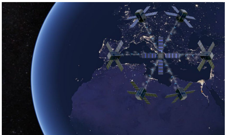
Figure 1 Artistic sketch of a hexagonal formation flight for the 16U4SBSP mission, beaming wireless electric power from space to a position on Earth.
