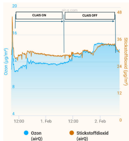
Figure 5: Left: 48h measurement of ozone and nitrogen oxide concentration, 24h with plasma (left, CLAIS ON), 24h without plasma (right, CLAIS OFF); Right: Log reduction of Staphylococcus epidermis (surrogate for MRSA)
