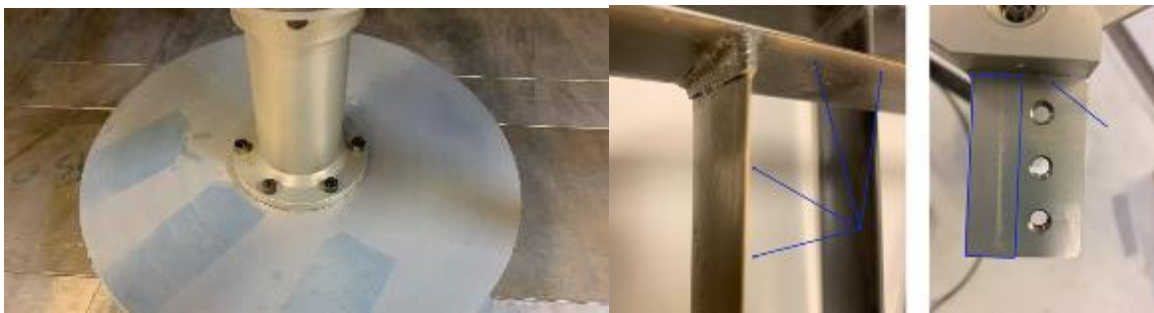
Figure 14. Dust deposition in different mechanical parts of the turbine.
