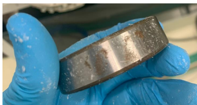
Figure 20. Corrosion detected in the bearings (COTS) produced by the CO 2 atmosphere.
