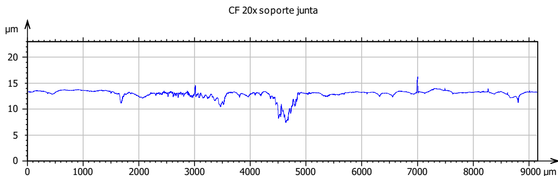
Figure 28. 2D roughness profile of the sealing mount after the test.
