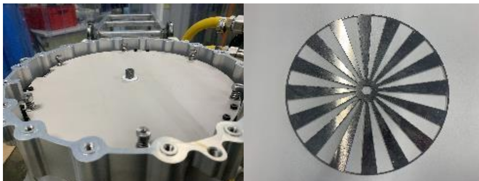
Figure 7. The vessel with holes for the enclosure, the preload springs, and the 4 TEG generators packaged and the DLC rotor.
