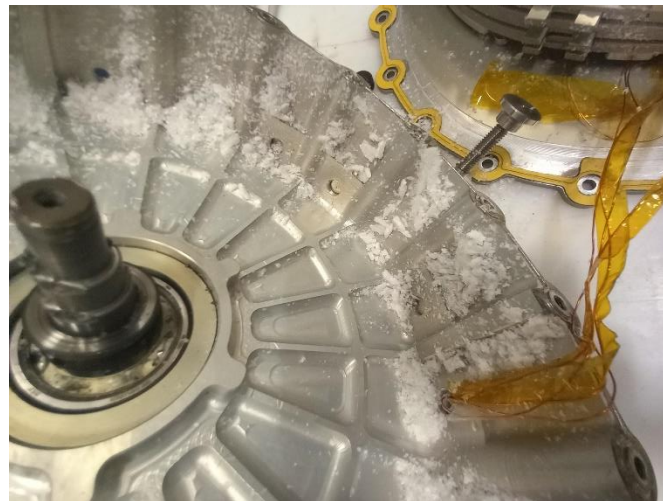
Figure 18. Presence of TFM parts in the vessel after the completion of the lifetime test campaign.
