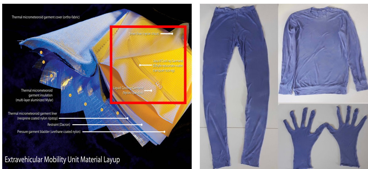
Figure 1 and 2: 1-Textile layers of NASA's EMU. Red rectangle indicates the aimed innermost layer of this project. These layers are mostly made of Nylon tricot; Nylon/spandex; Nylon/bladder. 2- AM1 treated Merinos textile body suit samples (BACT-021-HW1)
