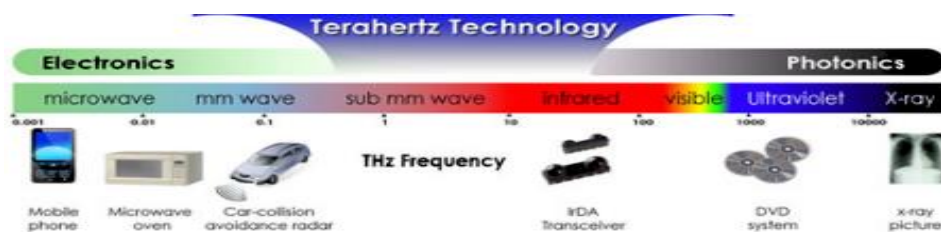
Figure 1 : Positioning of the terahertz domain in the electromagnetic spectrum
