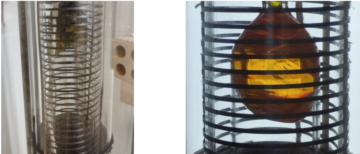
Figure 2 - First unsuccessful attempt to grow a crystal (left). A successfully grown crystal (right).
