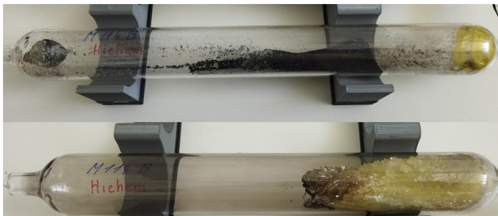
Figure 5 - Crystal from the original raw material (top) and the partially purified one (bottom)
