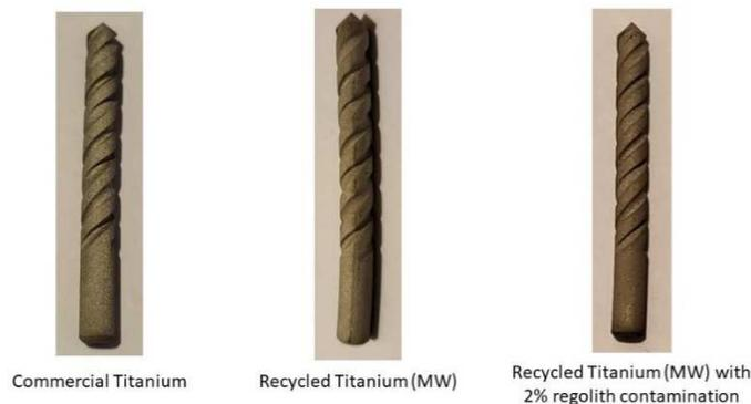
**Figure 7-6: Demonstrator parts printing: drill bit parts in all the different feedstock cases.**
