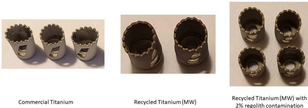
**Figure 7-5: Demonstrator parts printing: circular saw parts in all the different feedstock cases.**
