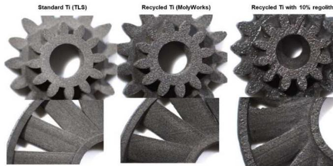
Figure 4-5: Ti green parts and the effects of the regolith contamination on the surface quality.
