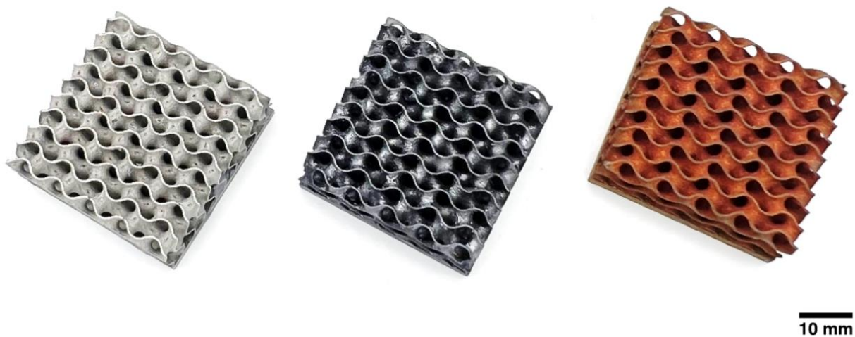
Figure 2: Gyroid heat sinks in three different materials, produced by LPBF. From left to right: Al-Cu alloy, Si-SiC, pure Cu.
