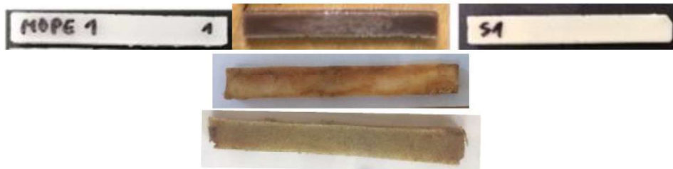
Figure 3-3. Examples for three-point bending samples with different chemical composition (pure MDPE, with Sulfur, with MGS-1 regolith)
