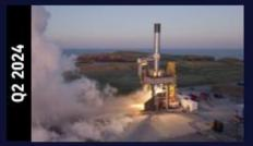
Fully integrated first stage with 9x engines
