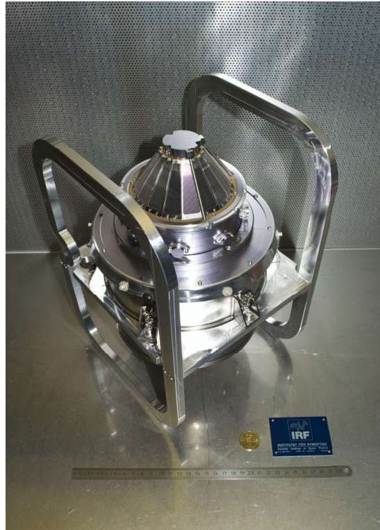
Figure 35 A photo of JDC with a coin and ruler for scale. The instrument consists of two cylinders on top of each other, topped by a cone. The handles around the instrument serve to ease transport and are not a part of the instrument. Credit: Philipp Wittmann, IRF Kiruna.
