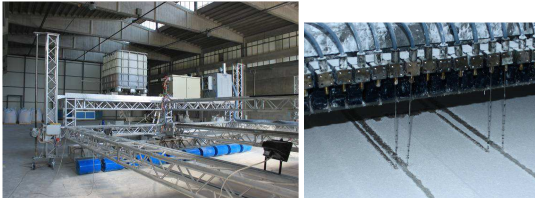
Figure 5.3 – The D-Shape system (left) and the printing head spraying the “ink” on the layer of sand (right).
