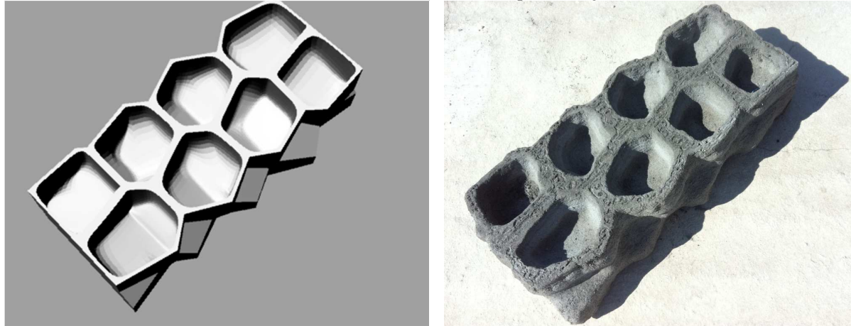
Figure 5.8 – Topologically optimised TDD1 STEP file closed cells structure (left, courtesy F+P) and the printed TDD1 obtained with Monolite UK D-Shape system(right)
