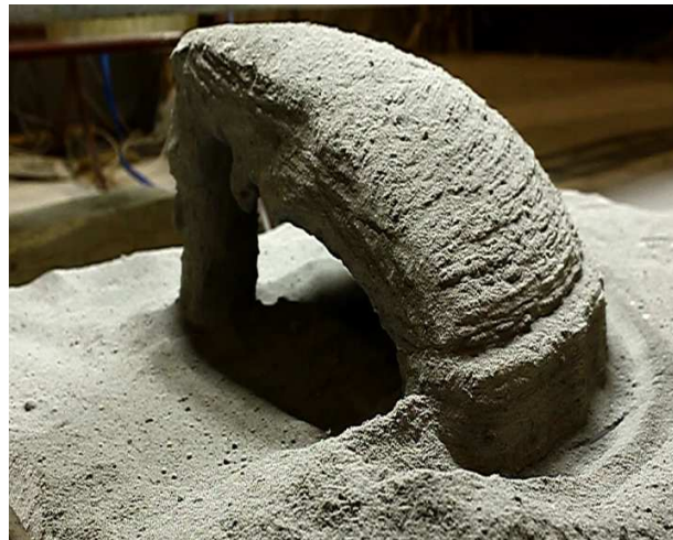
Figure 5.2 – Printing test with D-Shape system and DNA-1.
