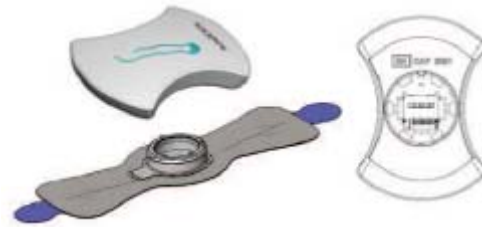
Figure 11: Mechanical casing and electrode patch.
