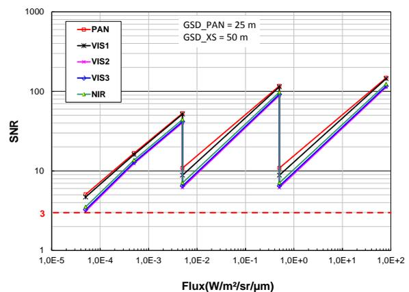
Figure 3.4-5: SNR values over the radiance dynamic for the 50 m option GSD XS
