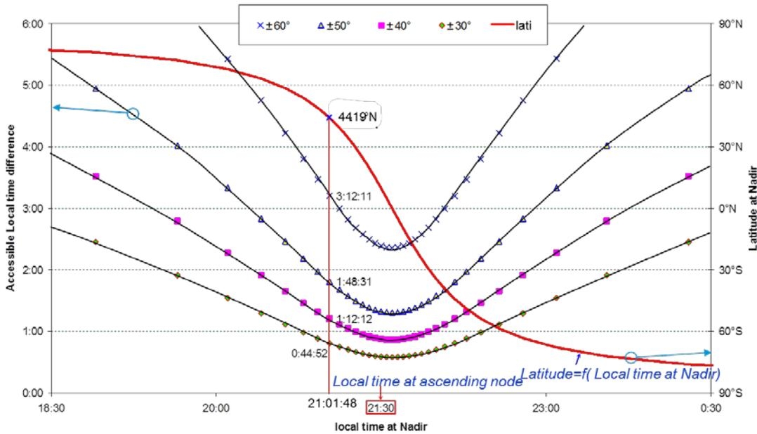
Figure 3.1-2: Accessible local time at target as a function of the off-track angle
