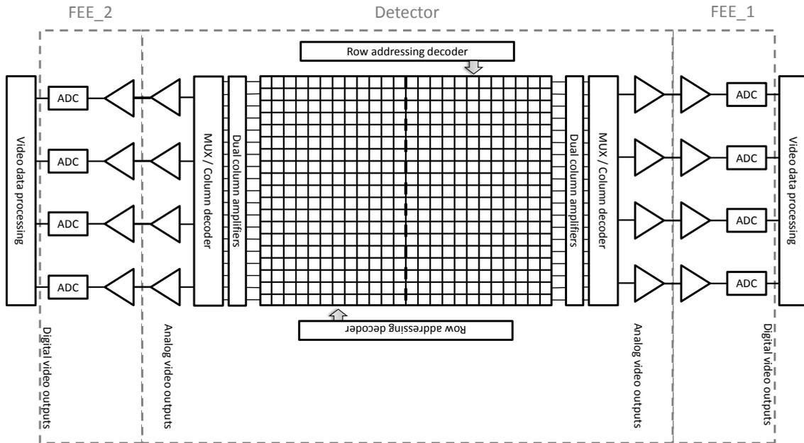
Figure 3.4-8: Detection chain block diagram
