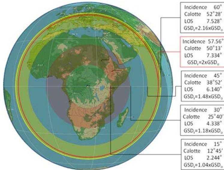
Figure 2.1-1: Observation from GEO Orbit, local incidence and GSD distortion
