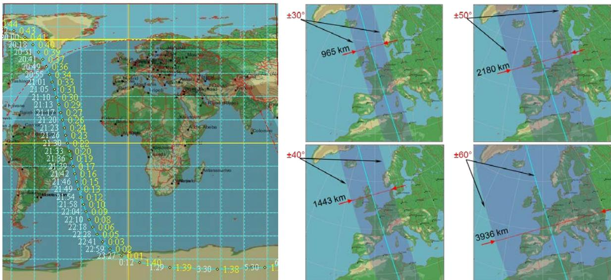
Figure 3.1-1: orbit and local time (left), access corridor and off track pointing over Europe (right)
