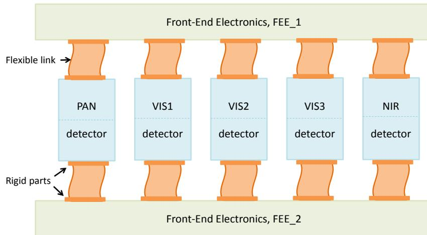
Figure 3.4-9: Schematic of the detectors / FEE modules assembly
