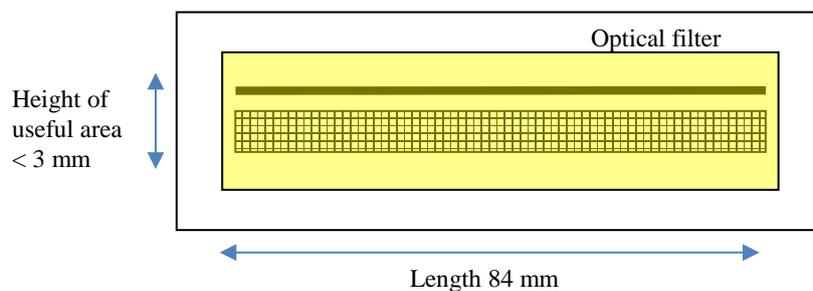
Figure 3.2-1: Detector with two sections: one TDI one single line with read-out line
