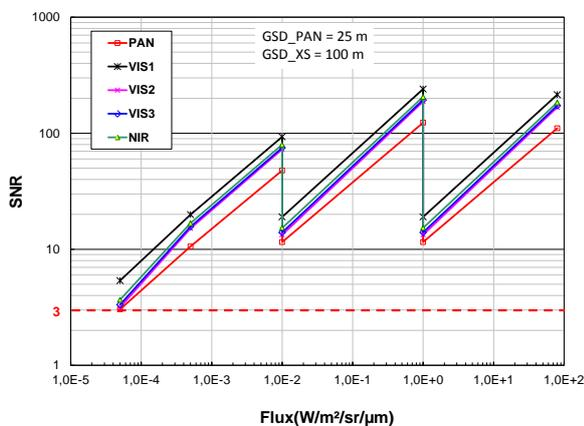
Figure 3.4-4: SNR values over the radiance dynamic for the 100 m baseline GSD XS
