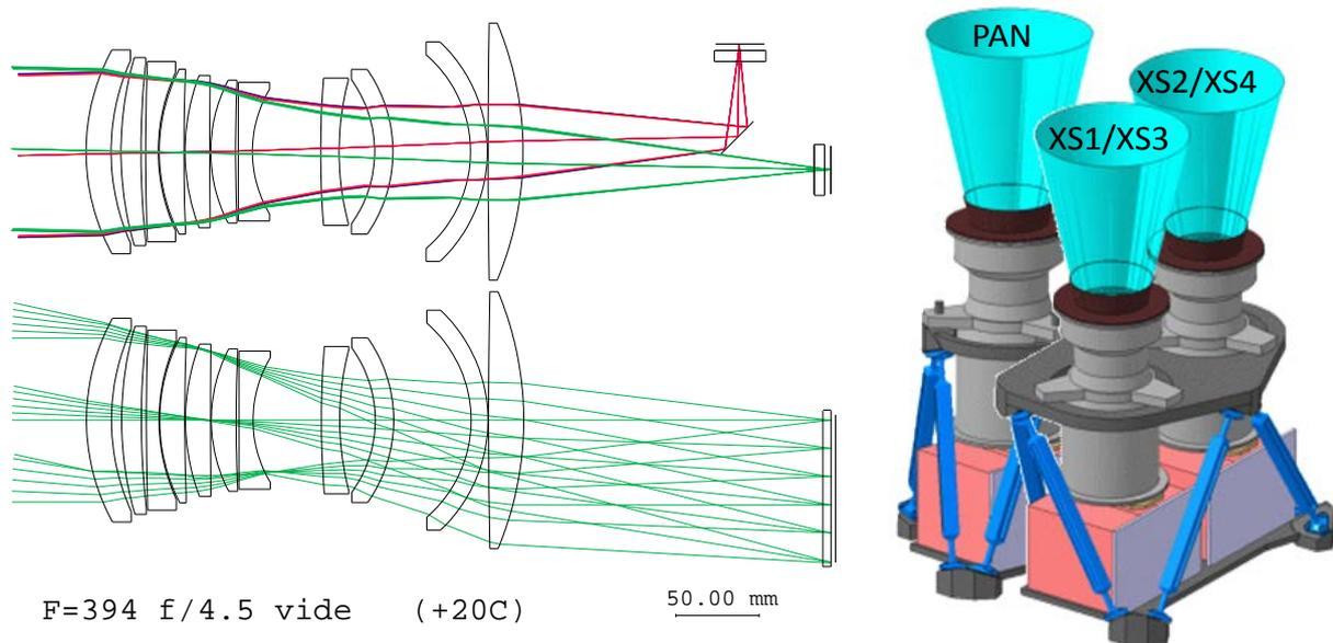
Figure 3.2-2: Pushbroom concept design. (Left) Dioptric lens at F/4.5 with two detectors. (Right) Lens arrangement without the scan/steering mirror, mechanism and structure.
