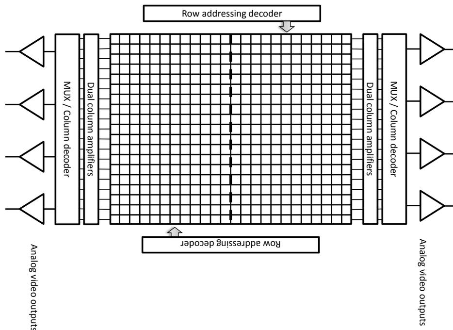
Figure 3.4-6: Detector block diagram with 8 analog outputs
