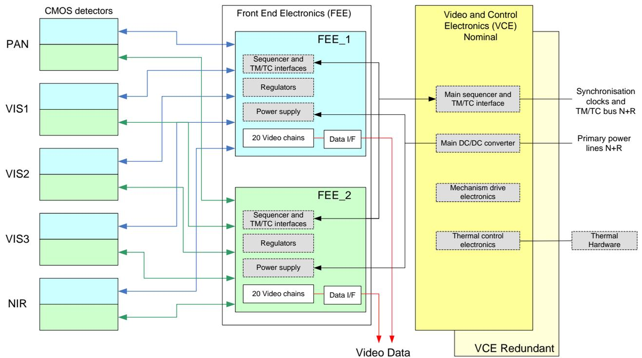
Figure 3.4-7: Detection chain architecture
