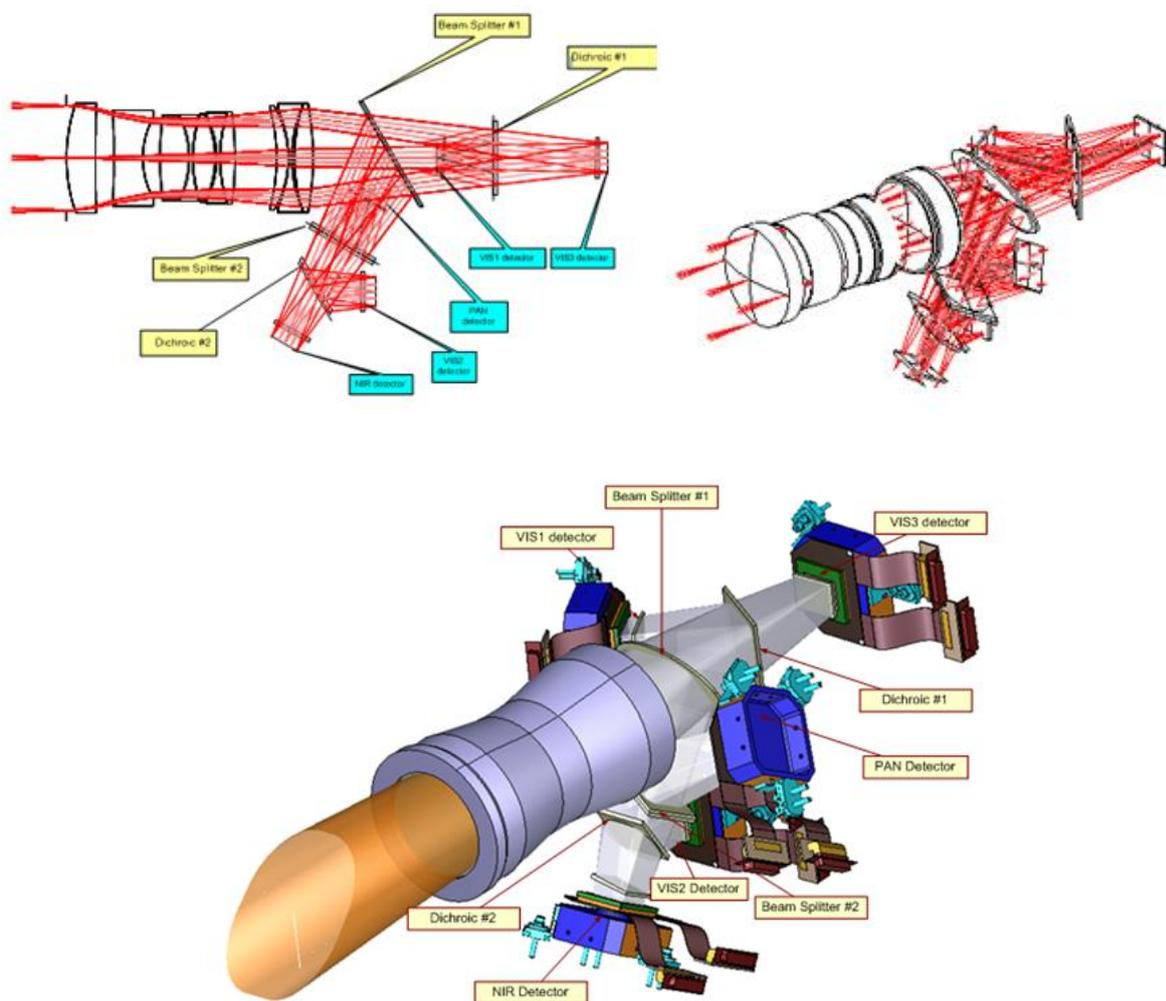
Figure 3.4-2: Different views of the NYX optical assembly
