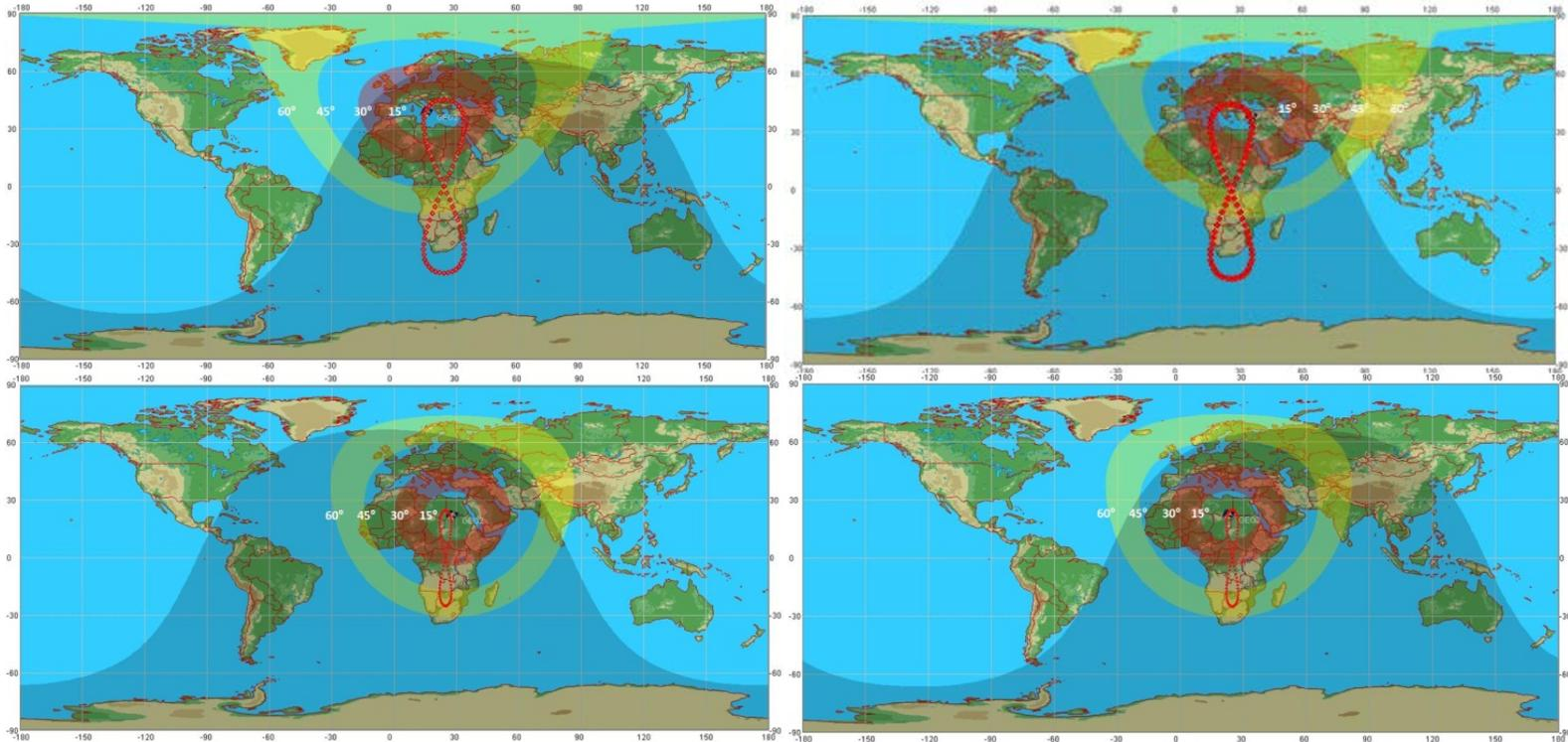
**Position of the satellite Nadir at beginning and end of the Sun avoidance manoeuvre ( $\pm 30^\circ$ )**
