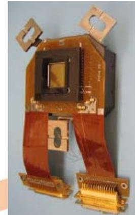
COMS/GOCI CMOS detector with 2 readout circuits and flex
