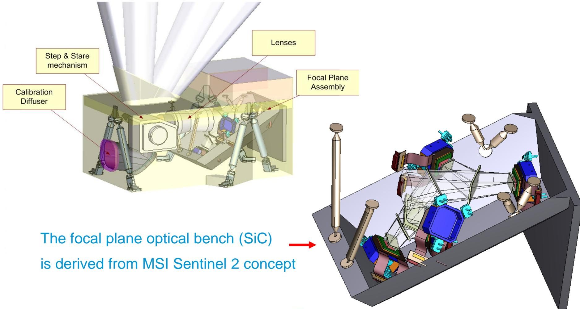
The focal plane optical bench (SiC) is derived from MSI Sentinel 2 concept
