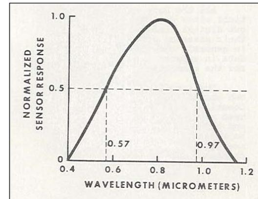
DMSP visible band spectral interval and normalized response curve(1974)
