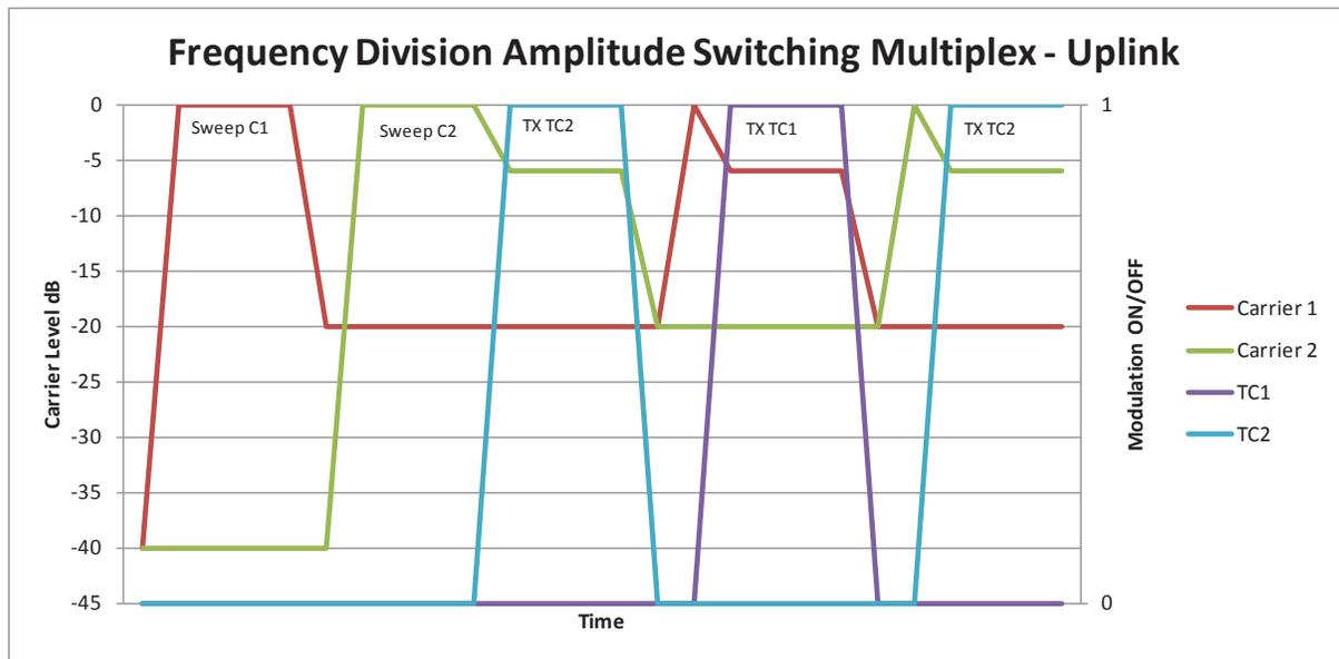
**Figure 2-1 Short Term Solution for MSPA using CFDMA with Amplitude Switching**
