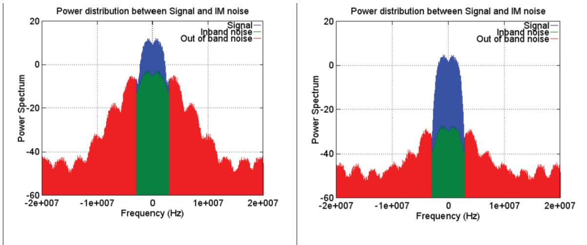
Figure 2-4 Two Carrier system with Non linear HPA
