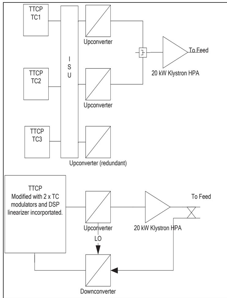
**Figure 2-2 Two options for implementing CFDMA Uplink (a) combining at RF before HPA without linearizer, (b) combining at baseband in DSP with DSP linearizer.**
