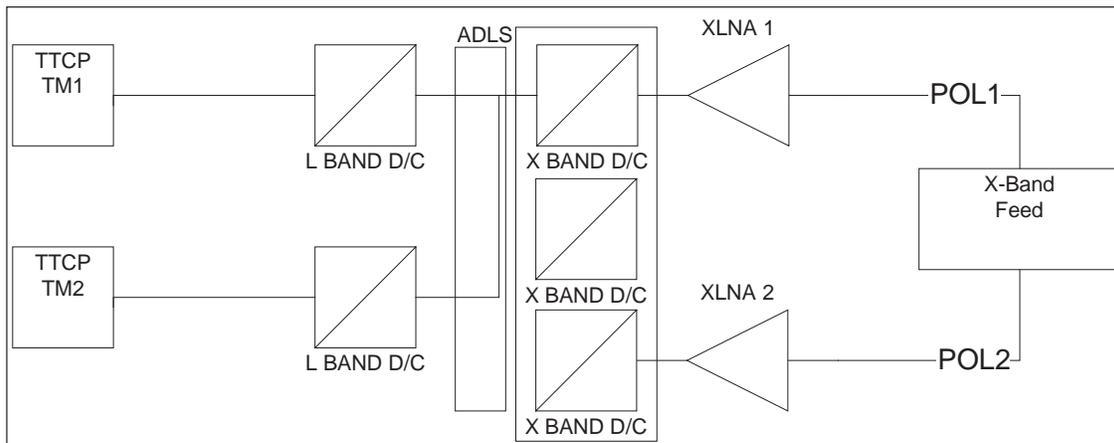
**Figure 2-3 DSA Configuration for implementing CFDMA Downlink.**
