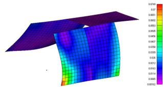
For what concerns the frame structure, it is pointed out that the margin of safety cannot be directly evaluated since a beam model was used with an "equivalent material" to represent a composite laminate. It turns out that the maximum stress in the frame is 566 MPa that is near to the ultimate strength of the Aluminium 7075 (~572 MPa) therefore further investigation should be done in order to assess the strength of the frame.
