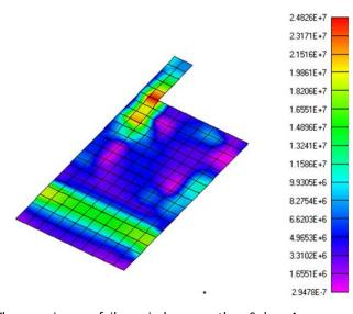
The maximum failure index on the Solar Array composite panel is 0.075 (well below the unit) therefore these components are able to survive to launch loads.
