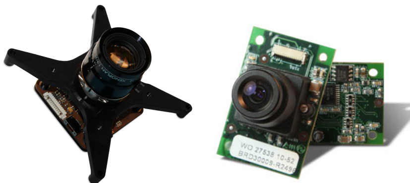
Figure 2: Camera Systems: Left, GomSpace NanoCam 1CU, Right: GumStix Caspa camera module
