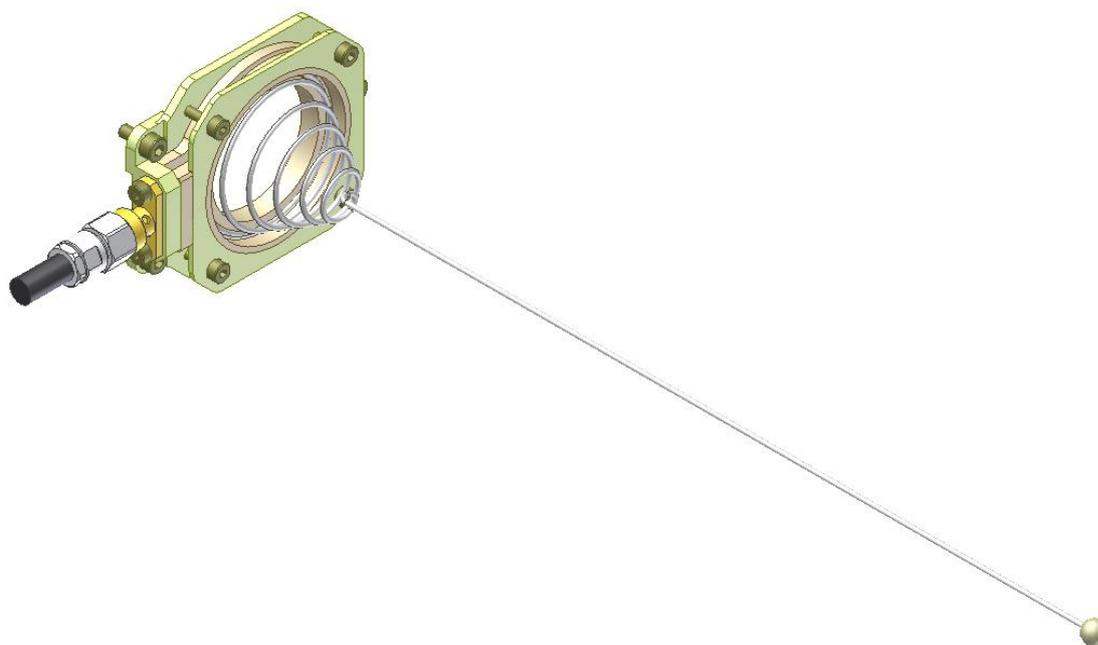
Figure 5-3 The Non-deployable Secondary Antenna preliminary design (Astronika)
