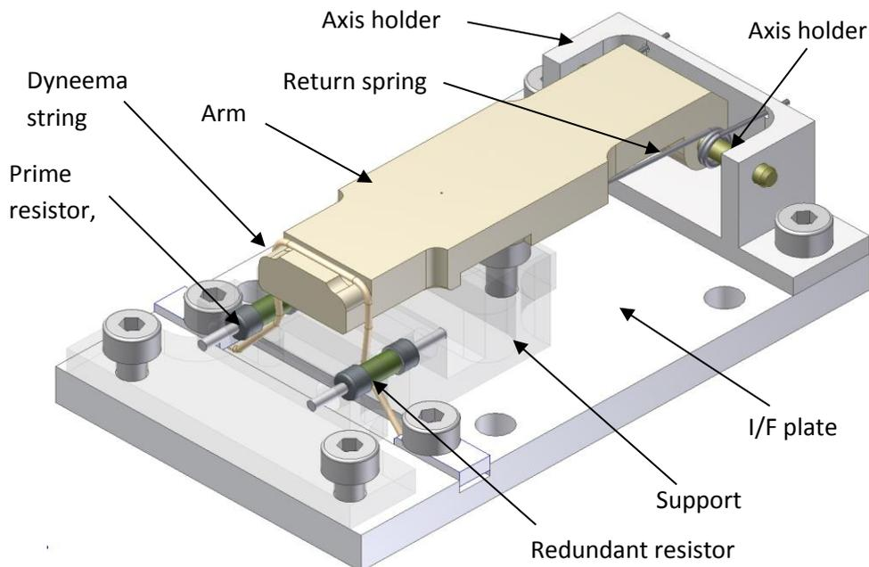
Figure 5-2 L&RM in closed position.
