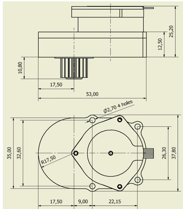
Figure 3-7 Dimensions in millimeters of the active damper
