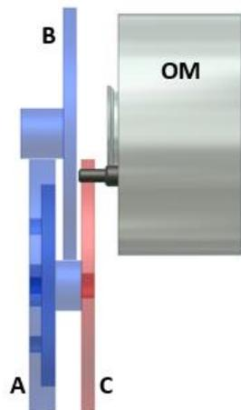
Figure 3-5 Oscillatory motor drive (OM): gear and the motor; **A** – outer spur wheel with interfaces to the hinge axis, **B** – mid toothed spur wheel with pinion, **C** – pinion with escapement, special toothed wheel, **OM** – oscillatory motor with four coils and pins engaged with the escapement wheel.
