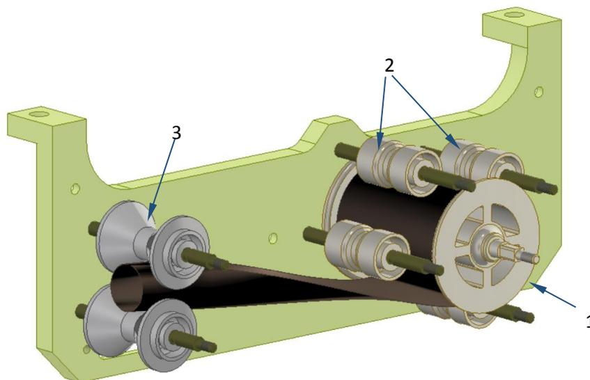
Figure 4-3 Main Antenna tubular boom guidance system:
