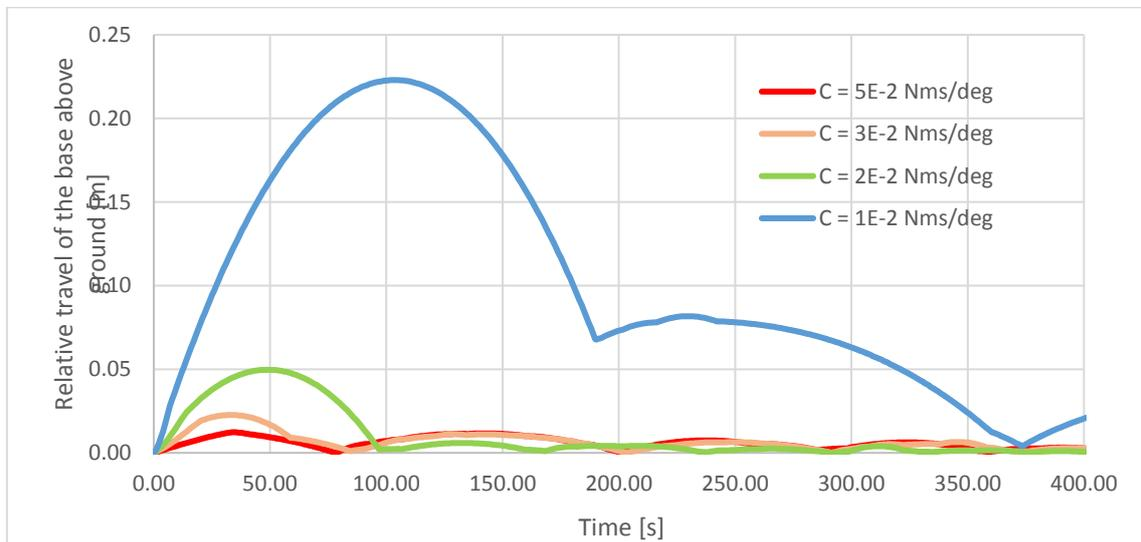
Figure 3-8, Relative travel of the base above ground [m] for various hinge damping constants
