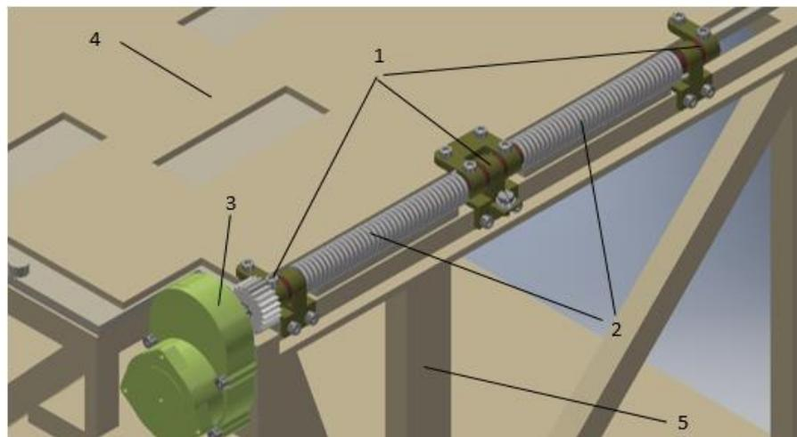
Figure 3-1 Overview of the hinge design
