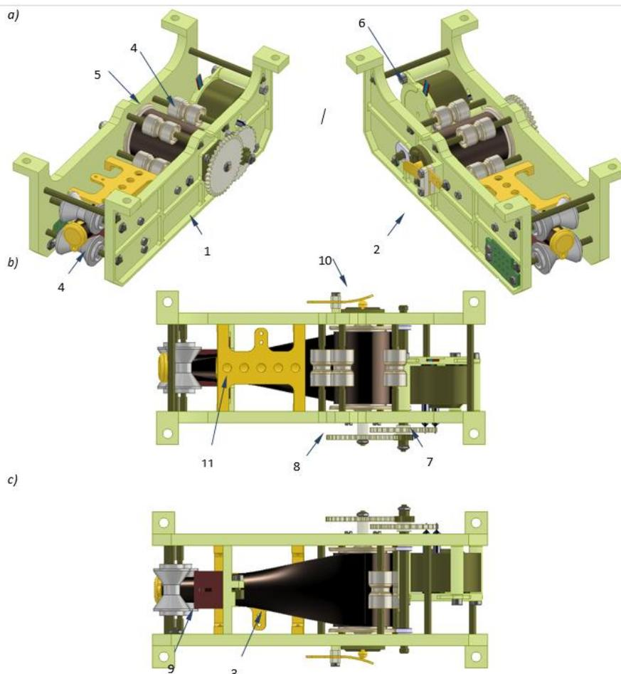
Figure 4-4 Main Antenna preliminary design: a) side isometric views, b) top view, c) bottom view: 1 – Right side wall, 2 – Left side wall, 3 – Tubular boom, 4 - Tubular boom guidance system, 5 – Storage reel, 6 – Oscillatory motor, 7 – Escapement mechanism, 8 – Gear (1:4 ratio), 9 - L&RM, 10 – Side spring for prime electrical connection, 11 – Connective rod for redundant electrical connection.
