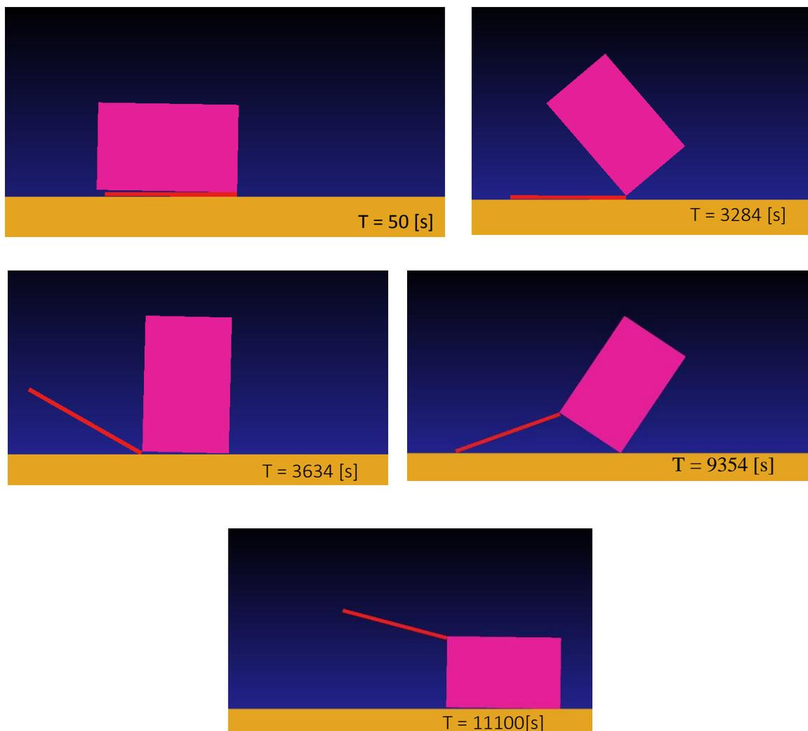
Figure 3-9, Deployment sequence from upside down configuration and hinge damping constant  $C = 2e1$  [Nms/deg]
