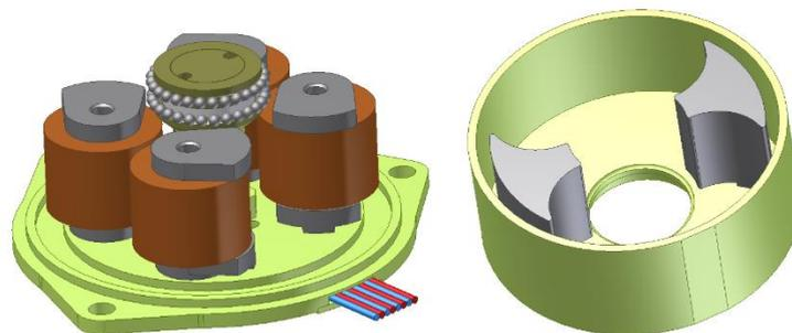
Figure 3-6 Left: Four electromagnets are fixed to the stator, in the upper central part is two row special angular bearing. Right: Rotor cup with two electromagnet's armatures – view from inside.
