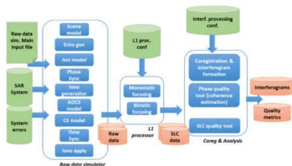
Figure 1 PSBSM architecture and interfaces
