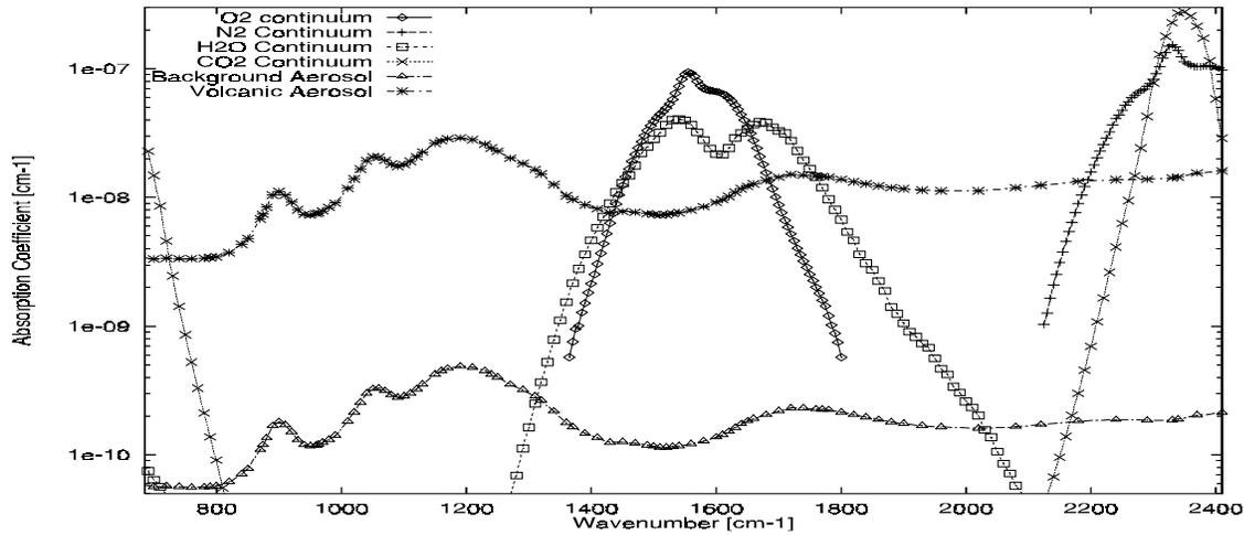
Figure 1. Typical values of the absorption coefficient of the different components of the atmospheric continuum in the middle infrared.
