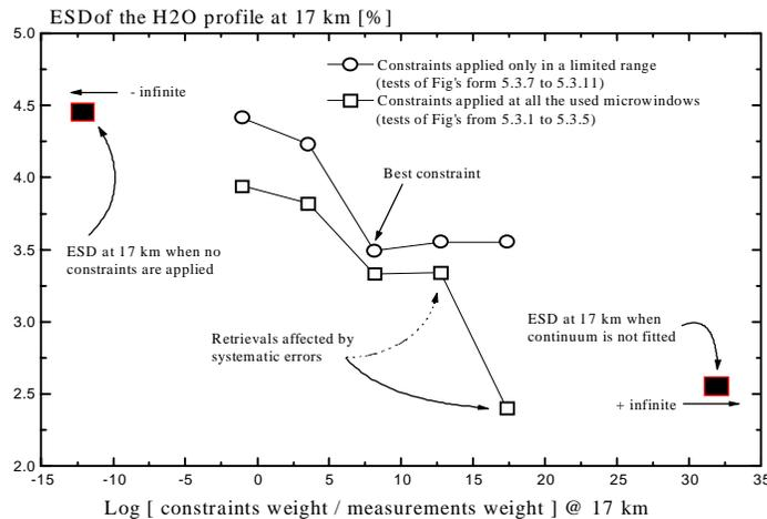
Figure 2. Variation of the e.s.d. of the retrieved volume mixing ratio of H<sub>2</sub>O at 17 km for constrains of different strength.
