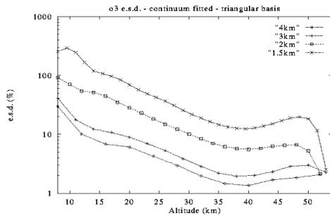
Figure 4. - The behaviour of the e.s.d. of  $O_3$  VMR versus altitude for vertical sampling steps of 1.5 km, 2 km, 3 km and 4km
