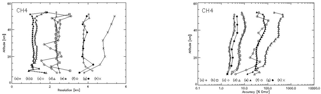
Figure 12. - Resolution (right) and Accuracy (left) of the CH<sub>4</sub> retrieval in cases a) and b) to h).
