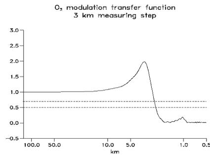
Figure 3. Example of Modulation Transfer Function for measuring/retrieval steps of 3 km
