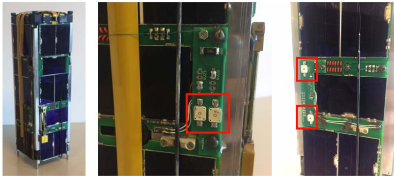
Figure 15 - LED mounting on Ursa Maior CubeSat [RD-05]
