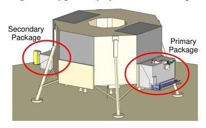
The Primary Package carries the carbo-thermal reduction payload, which extracts oxygen from the regolith and produces water; the internal layout is shown below.
