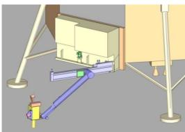
Each package includes a robotic arm which, for the oxygen extraction payload, is dedicated to the excavation of regolith and, for the volatile prospecting payload, carries the instrument in proximity of the surface for operations. The surface area reachable by each arm is about 2.4 m<sup>2</sup>.
