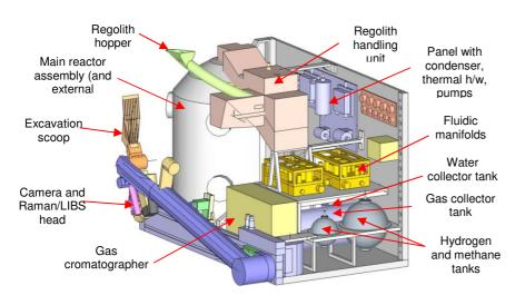
An important part of the effort has been devoted to trade-off. definition. sizing and analysis of the carbo-thermal reactor, the core element of the ISRU Payload. The reactor operates in a batch mode; it is loaded from the upper side with regolith filling (about 1 kg); discharge of spent regolith occurs by gravity from the lower side, to the lunar surface; for these functions a system of
