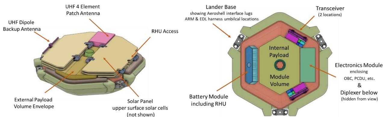
**Figure 7. (left) Stowed lander (right) Internal equipment and payload volume**
