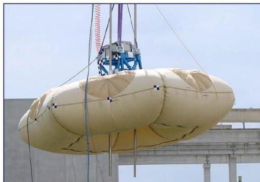
**Figure 4. 2013 ExoMars Mission - Airbag Prototype tested at Aero Sekur**
