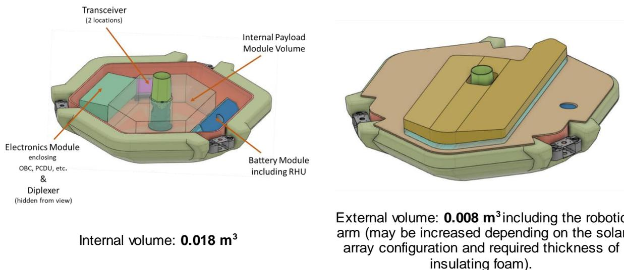
**Figure 10. Internal (left) and external (right) payload envelopes and volumes**
