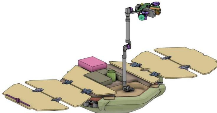
**Figure 9. The fully deployed lander with the robotic arm in the mast position**
