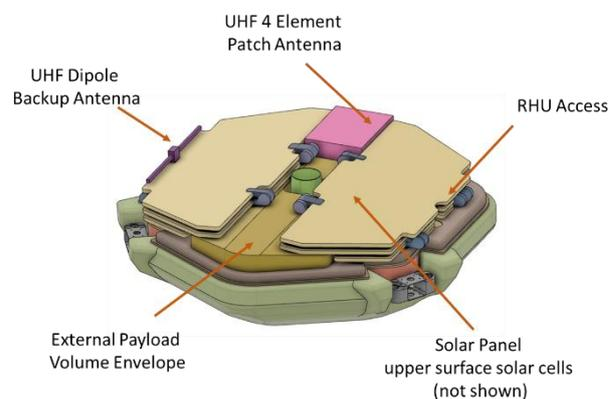
**Figure 3. (left) The pocket watch configuration of the Beagle 2 lander (right) The cabriolet configuration with solar cells and UHF antenna available in the post-landing configuration.**
