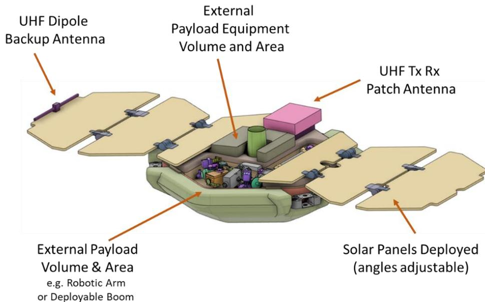
**Figure 8. Lander with solar arrays deployed (prior to deployment of robotic arm)**
