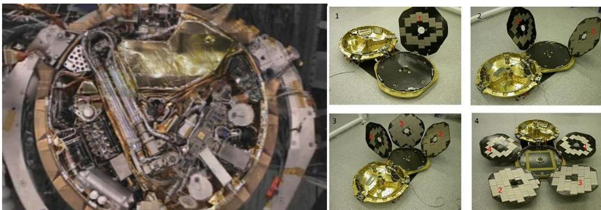
Figure 2. (left) The lander base containing all functional elements of the lander, the internal payloads and the robotic arm. (right) Solar Panel deployment sequence
