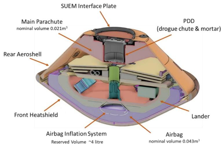
**Figure 6. The probe including toroidal airbag and parachutes**
