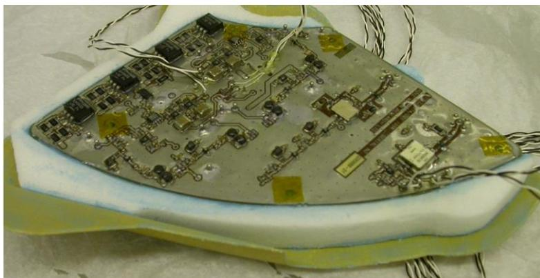
**Figure 5. The Beagle 2 Radar Altimeter Trigger (RAT)**
