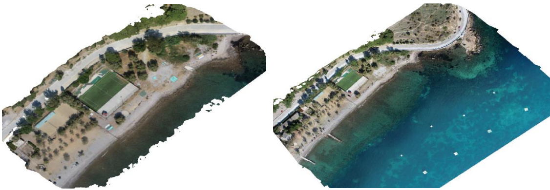
Figure 3 Orthorectified UAV data collected over the plastic targets in Mytilini (Lesvos Island, Greece)
