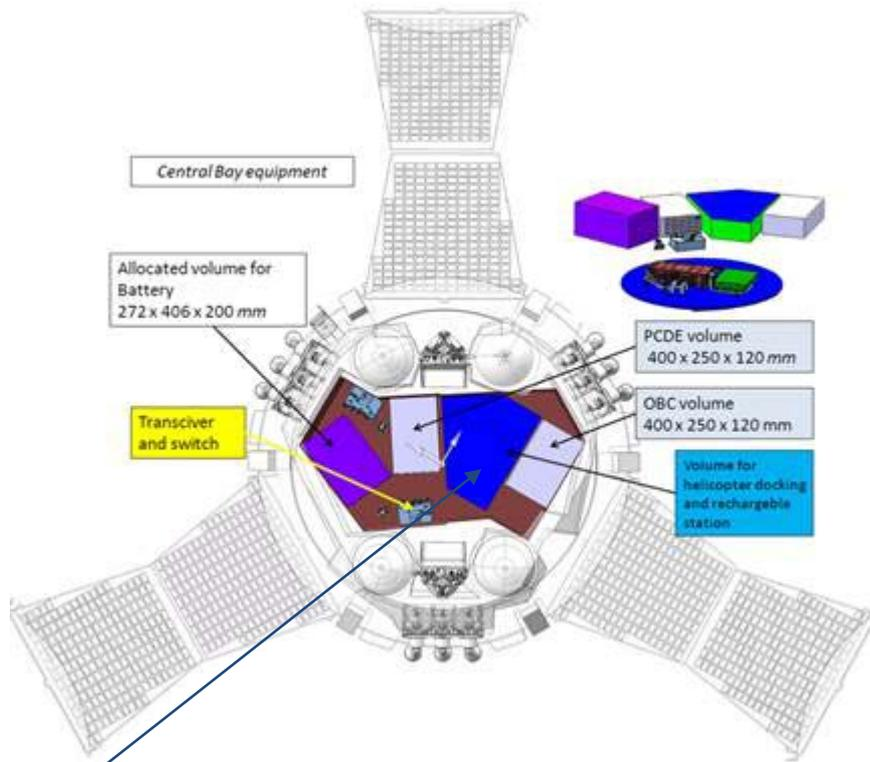
Figure 2-16 MSPC Surface platform Configuration layout
