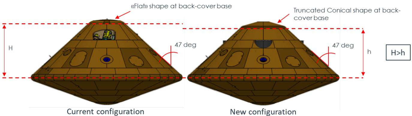
Figure 2-8 Left: EXM configuration; Right: MSPC Aeroshape difference driven by new PAS shape and dimensions
