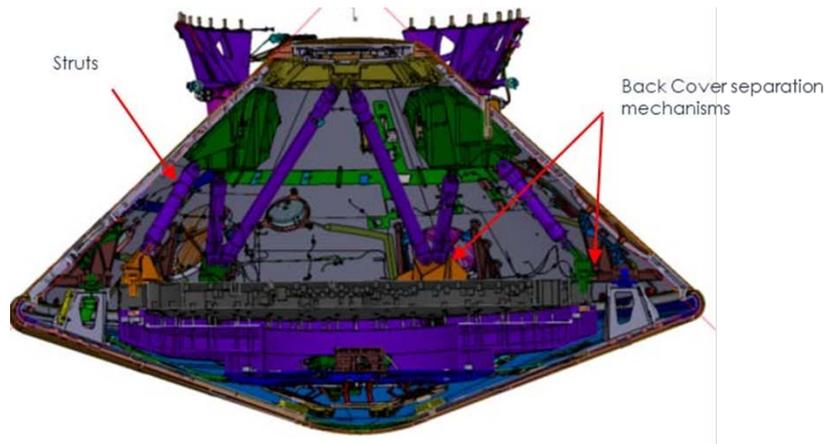
Figure 2-4 EXM EDM Struts
