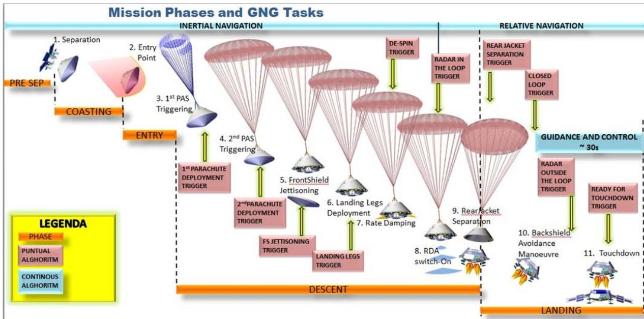
Figure 2-12 Schiaparelli EDL GNC Design – Phases, Events and GNC Modes
