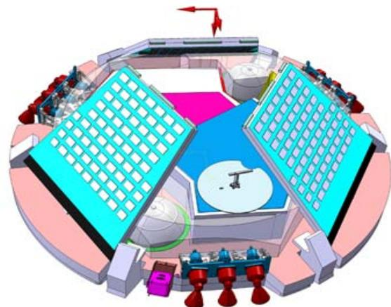
Figure 2-13 **MSPC Configuration with deployed SA (left) and stowed SA (right)**
