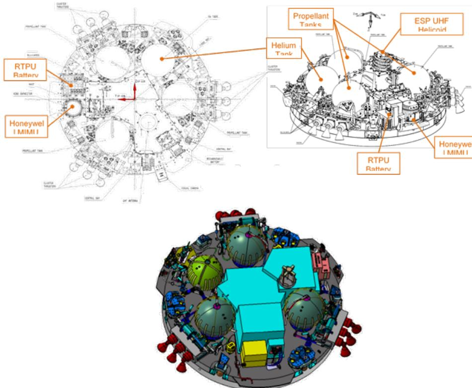
Figure 2-15EXM EDM-Schiapparelli Configuration layout
