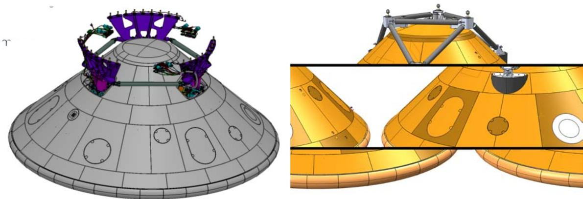
**Figure 1-1** *Left: EXM EDM “Schiaparelli”, Right: EDM review as result from the MSPC study. The exercise of reconfiguration has been carried out keeping the EXM EDM lander sizing (same diameter of the platform)*
