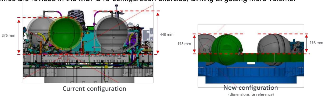
**Figure 2-9Left: EXM EDM RCS configuration; Right: new accommodation of tanks, obtained by cut-outs in the Surface Platform**
