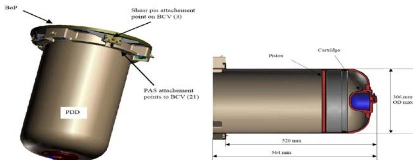
Figure 2-6 EXM EDM PAS design
