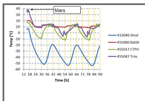
Figure 2-10 Typical temperature trend with capacitor at 12 °C
