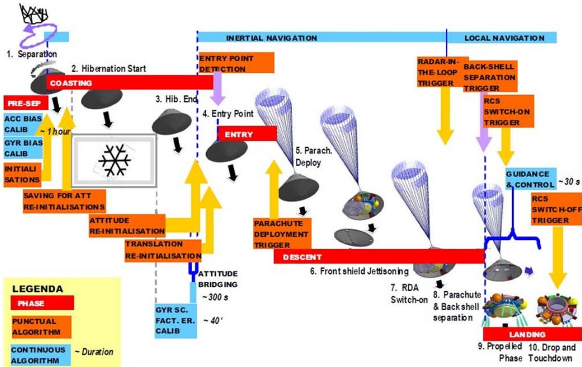
Figure 2-11 Schiaparelli EDL GNC Design – Phases, Events and GNC Modes
