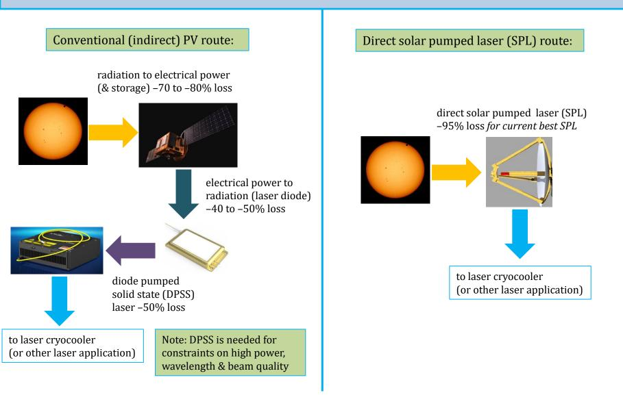
The use of an SPL **avoids 2 conversion losses**, i.e., radiation  $\rightarrow$  electrical, and electrical  $\rightarrow$  back to radiation
