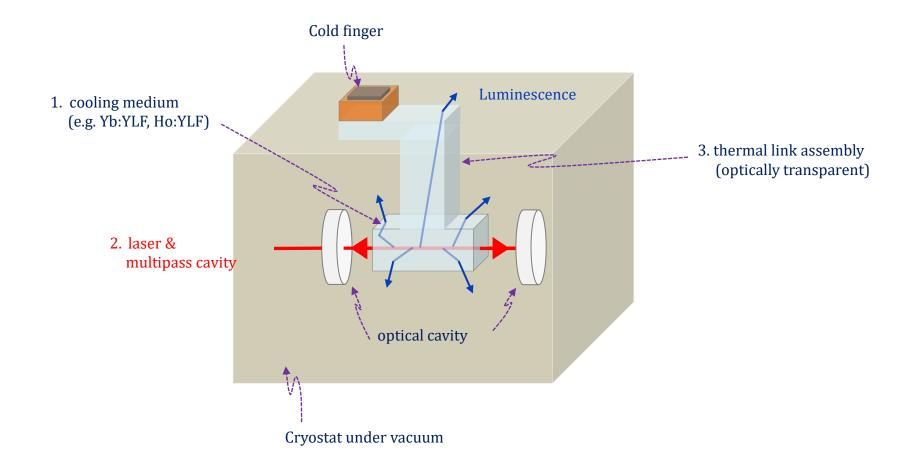
Optical cryocooling is the *only* stand-alone and active cryocooling technology that is fully free from micro-vibrations, due to absence of moving parts *and* moving mass.
