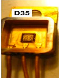
Figure 2 - Flight Qualified Schottky Diode (delidded) for BepiColombo and other ESA Mission. Image: Godignon et al., Alter Technology Group.
