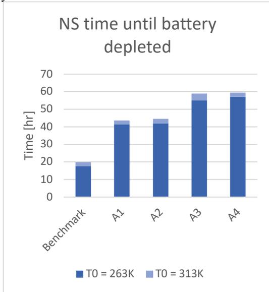
Figure 11 – (Short Polar) Night survival time for the various architectures
