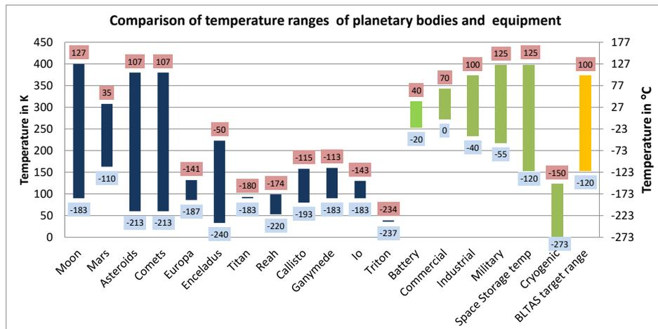
Figure 1 - Comparison of temperature ranges of planetary body surfaces and electronic equipment
