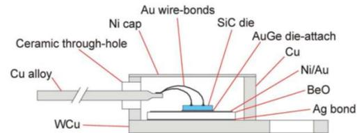
Figure 5 - Cross section schematic of TRL8 Schottky diode packaging qualified for 103K to 543K (-170C to +270C). Image: Godignon et al., Alter Technology Group.
