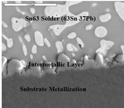
Figure 4 - Formation of intermetallic compounds in soldering. Image: Indium Corporation.
