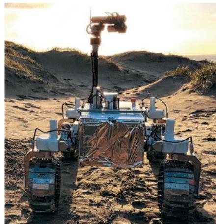
*Figure 8 – LUVMI Rover early prototype*
