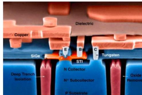
Figure 3 - SiGe HBT construction Image: Cressler, Georgia Institute of Technology
