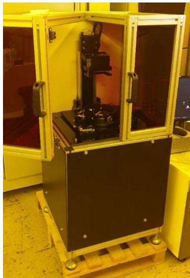
Figure 5.3 – Prototype of LCM machine with reduced size and weight.
