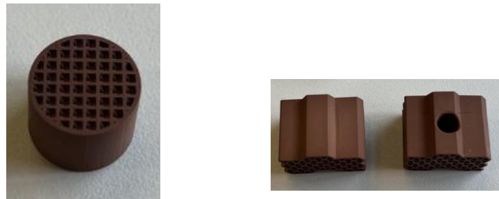
Figure 7.1 – Demonstrators parts realized (filter mesh on the left, brick on the right).
