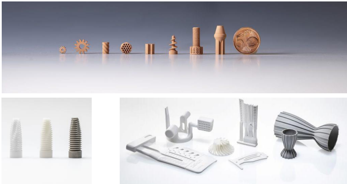
Figure 3.1 – Potential lunar regolith (on the top) and different materials (on the bottom) demonstrator parts for life-support systems in a future lunar outpost.
