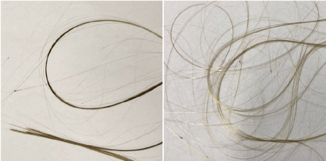
Fig. 1: LMS-1 – Bundles of LMS-1-M-1L fabricated with the single tip bushing. Size approx. 25 cm (left) and 10 cm (right).
