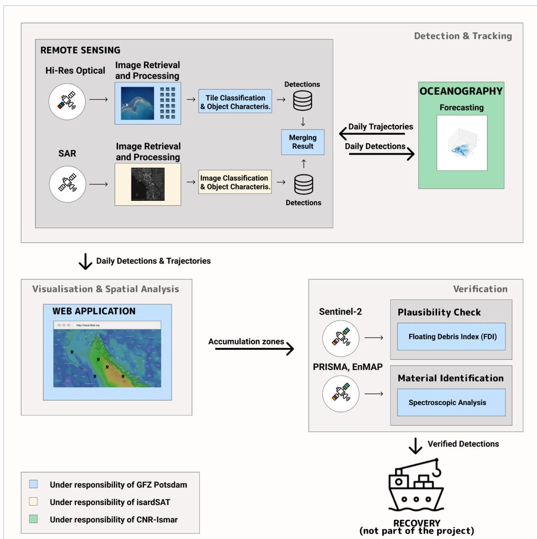
**Figure 1:** General idea and concept of the TRACE system showing its components, their interplay, and the data processing flow on a general, abstracted level
