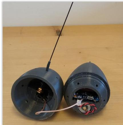
*Figure 9:3D model of the tag with the electronics.:*
