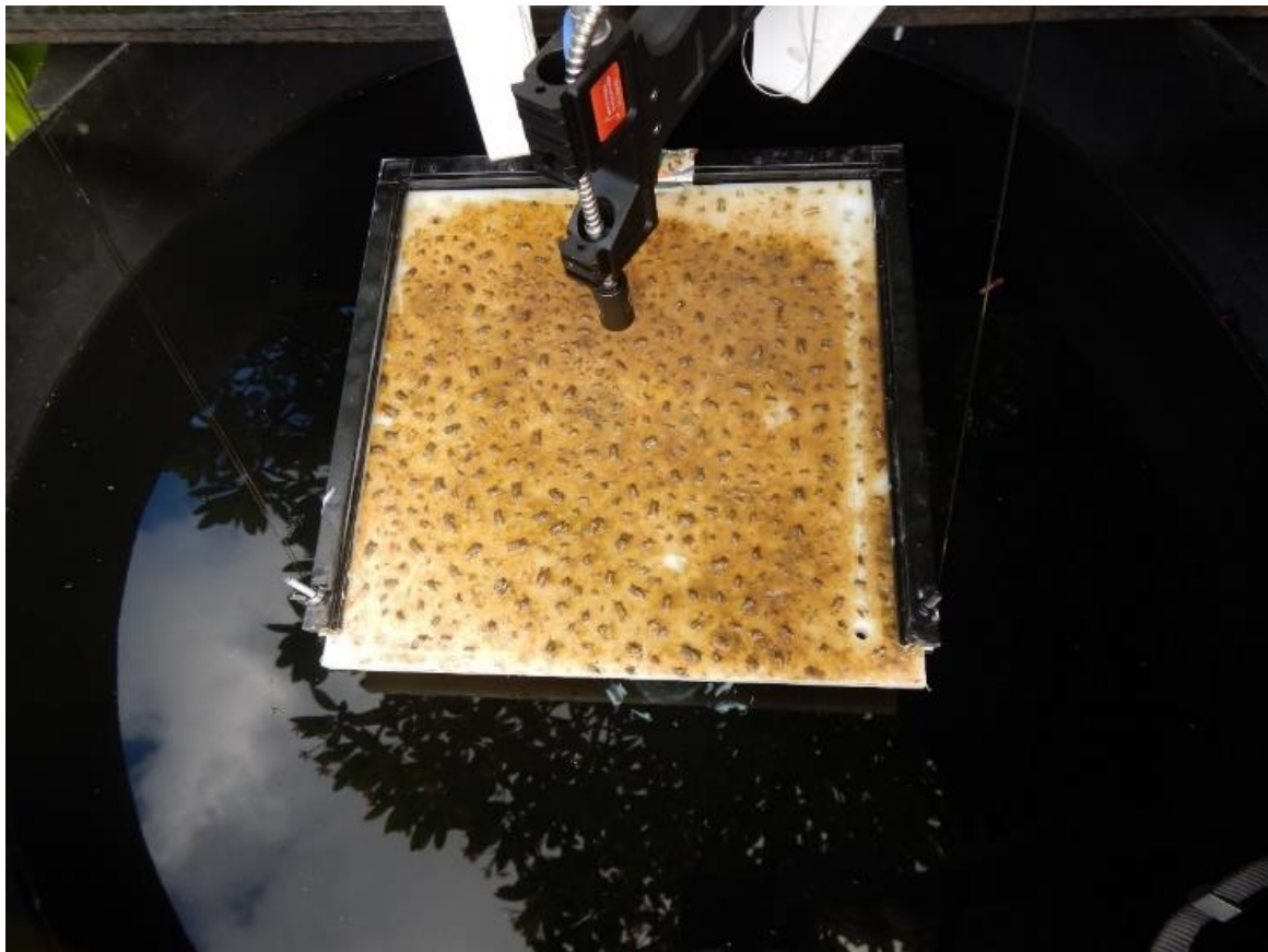
Figure 4: Close-up of the measurement setup using a similar clamping setup as the indoor lab measurements. The spectroradiometer lens is visible at the top of the image, pointing perpendicular to the biofouled sample.
