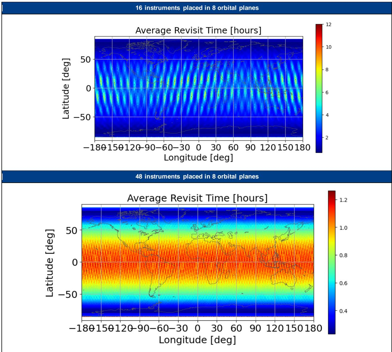
**Figure 4-1: Average Revisit Time over the entire globe after 1 day for the two configurations**
