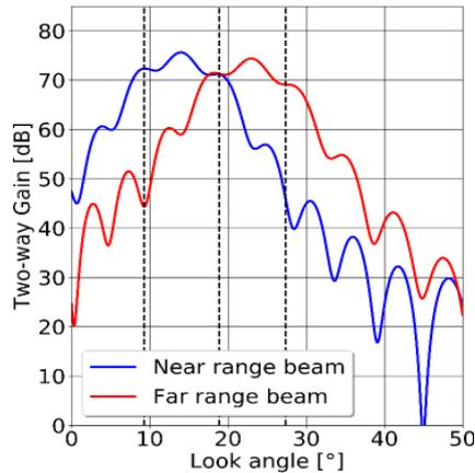
**Figure 5-4 Achieved sector beams as function of look angle. The look angle span between the near range and the far range is highlighted for each beam.**
