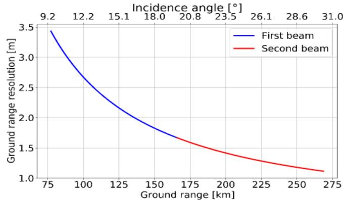
**Figure 5-3 Ground range resolution as function of the ground range for the two beams.**
