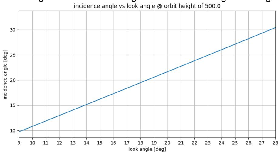
**Figure 5-2 Incidence angles as a function of look angles for an orbit height of 500.0 km.**
