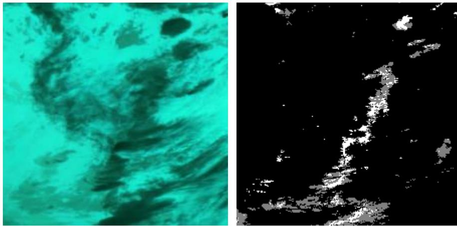
**Figure 6-1** Sample input image from SIVIRI and its corresponding GT from OPERA.
