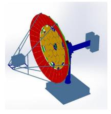
The COMPASTA toolset has been evaluated on the CONTEST case study [RD19], a case study from the energy domain. The case study concerns the co-generation of electric and thermal energy, using a solar concentration made up by a dish, plus a stirling engine. The system can be subject to faults (e.g., engine errors, dish over-heating) and must satisfy several functional and safety requirements (e.g., automatic shutdown in case of unrecoverable errors).
