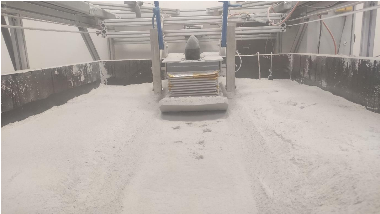
Figure 3. Dusty environment of the work with regoliths. Particulate matter concentration in the lab room always exceeded safe values. Tests always need to be performed in full personal protective gear.
