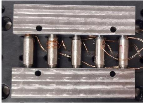
Figure 2 – Photo of the assembled manifold
