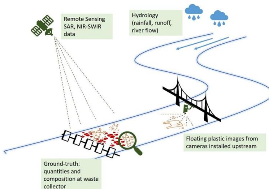
Figure 1 - Concept of "Plastic Monitor" experimental setup in the Indonesian river.
