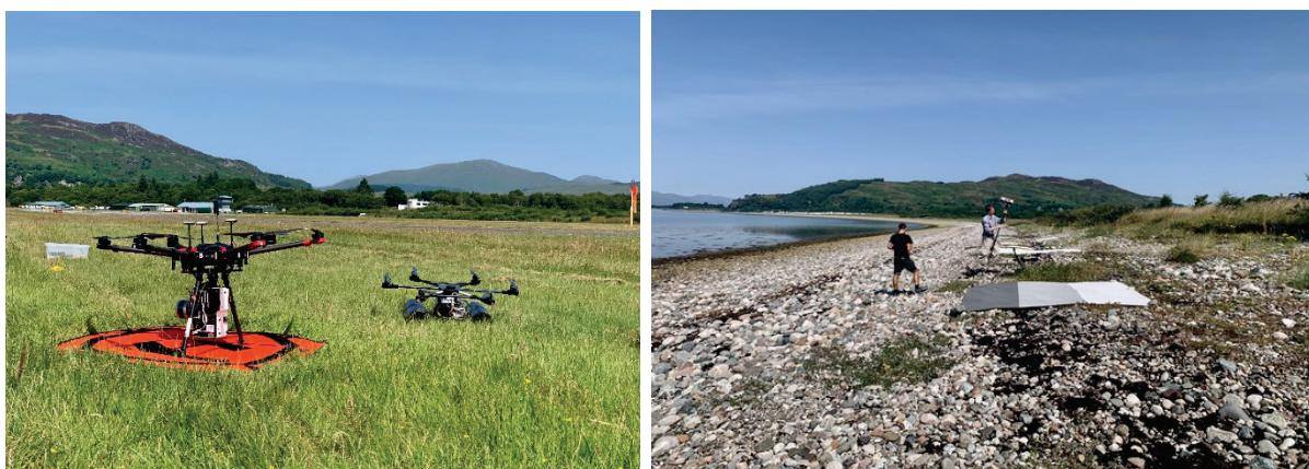
**Figure 1:** Left: Headwall (larger) and BaySpec (smaller) hyperspectral sensors mounted in RPAS at Oban Airport. Right: target deployment on the shore and SVC being operated.
