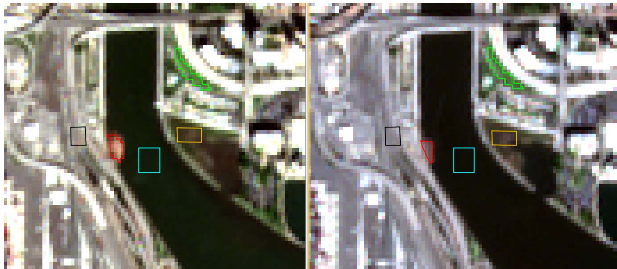
Figure 11: Natural colour Sentinel-2 (L2A) image of a Garbage Boom on the LA River on the 23/02/2017 (left) and 05/03/2018 (right). Natural colour RGB (Band 4 / 665 nm, Band 3 / 560 nm, Band 2 / 490 nm). Coloured polygons indicate pixels used to describe reflectance values of each surface type. Black = Urban, Red = Litter, Blue = Water, Green = Trees, Yellow = Grassy Lagoon. Source: Copernicus hub.
