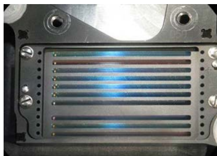
Figure 27: Sentinel-2 MSI VNIR detector with stripe filters associated to 10 spectral bands
