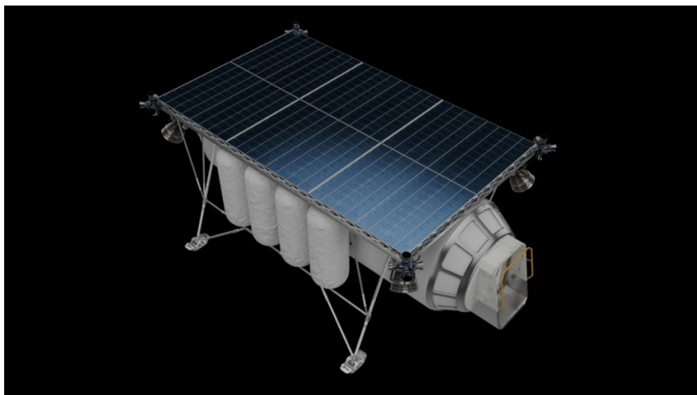
Figure 40: Astrostrom's concept of Lunar Landing Gantry with a factory module attached underneath.
