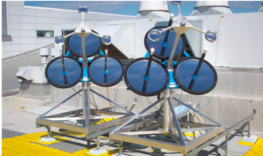
Figure 53: Ground test model of the Optical Waveguide (OW) solar energy system (Credit: Nakamura)
