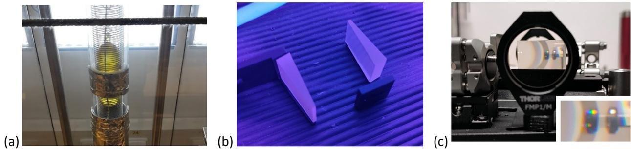
**Figure 4:** (a) Furnace during crystal growth. (b) A pair of wedges under UV illumination. (c) One wedge of Calomel, mounted in the interferometer; note the chromatic aberration due to the prism-shape of the crystal, and the double image of the screw, due to its birefringence.
