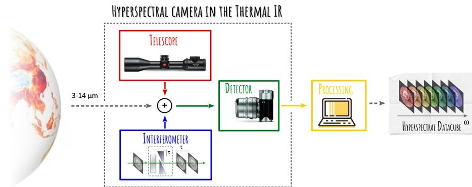
Figure 2: general scheme of a hyperspectral imager operating in the Thermal infrared.
