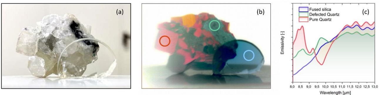
Figure 8: thermal imaging of a sample heated at 200°C. (a) The sample in the visible spectral range. (b) False-RGB image in the thermal infrared, obtained with the innovative hyperspectral camera developed in the project. (c) Emissivity spectra at selected points.
