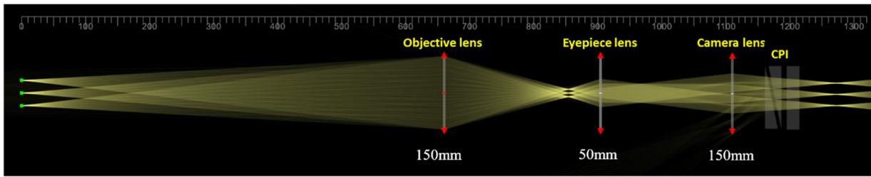
Figure 6: Design of the optical scheme of the telescope. CPI: our interferometer.
