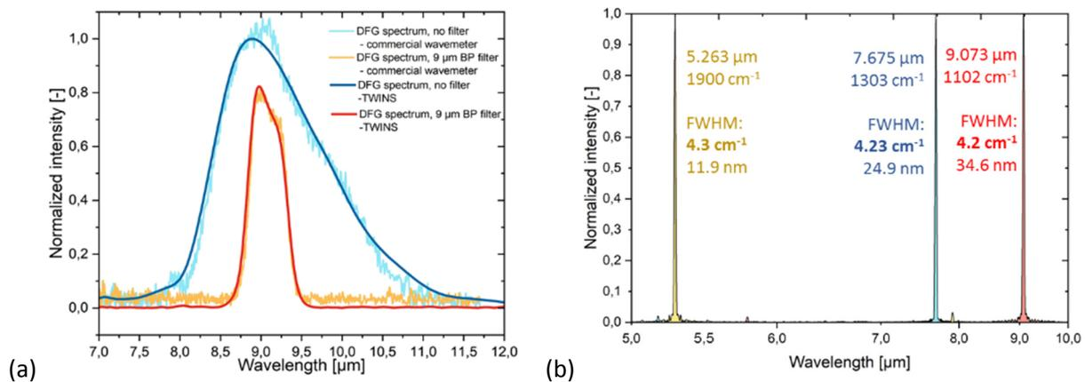
**Figure 5:** Spectral characterization of our interferometer. (a) Measurement tests of a light beam. Thick lines: spectra obtained with our novel interferometer. Thin lines: spectra obtained with a commercial spectrometer. (b) Spectra of monochromatic lasers.
