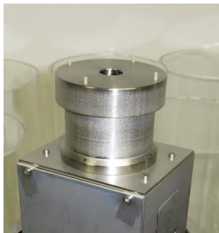
Figure 3-2. The assembled thruster prototype
