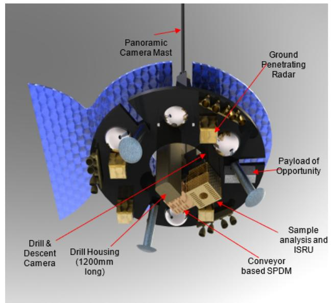
**Figure 3-4: Lander Payload Configuration Overview Concept**
