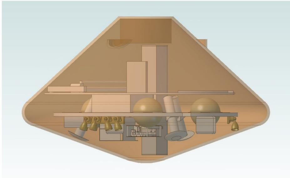
**Figure 3-2 Lander Stowed in Aeroshell Side View**
