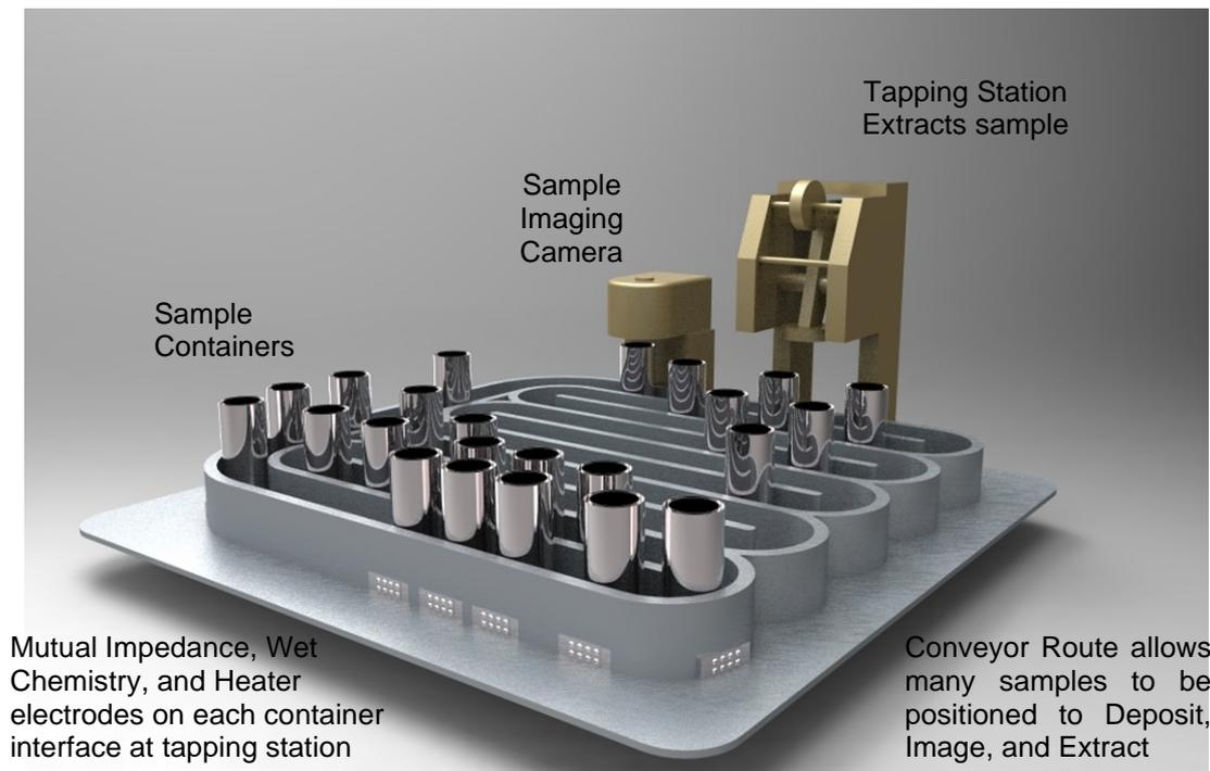
**Figure 3.6. SPDM concept CAD – conveyor option (Baseline)**
