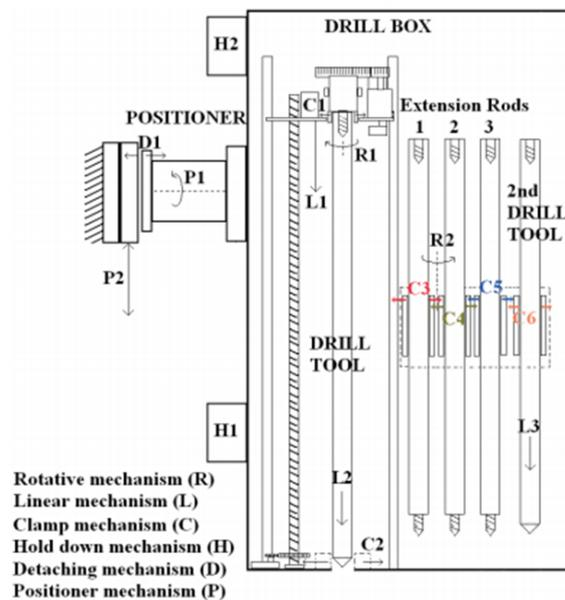
**Figure 3.5. Proposed drill mechanism schematics**
