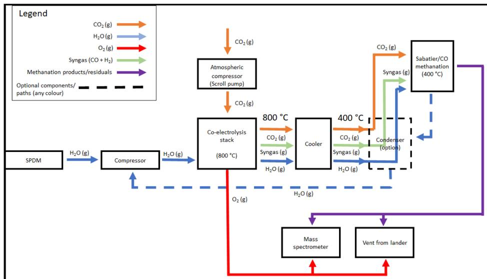
**Figure 3.7. Baseline ISRU processes within the DRUM**
