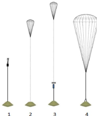
**Figure 3-3: Parachute Deployment Sequence**
