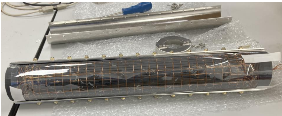
Figure 3-1: The wound coil former is positioned within the first section of the internal passive shield (below), which is subsequently sealed with the second section of the shield (above) prior to testing.
