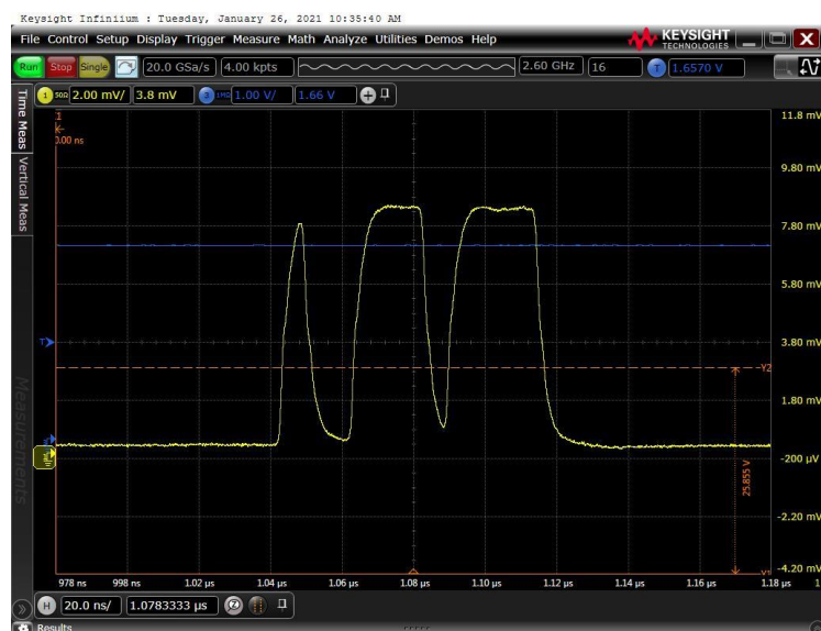
Figure 5: Intensity modulated output of the PIC
