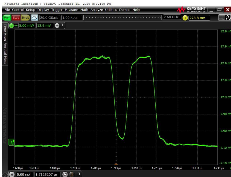
Figure 3: Oscilloscope trace of a current waveform generated by the control electronics (5 ns/div).
