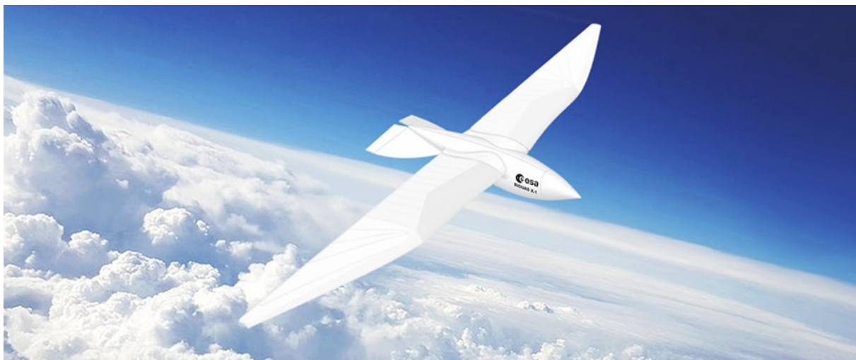
Figure 14 – Concept image of final project demonstrator prototype as an unpowered aerosonde glider
