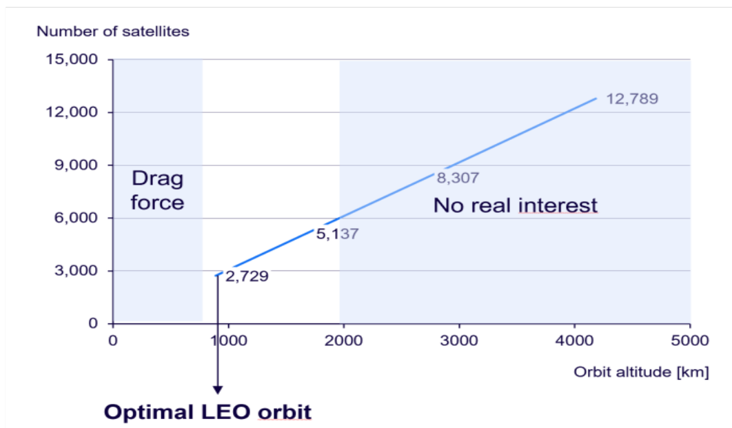
Figure 3 - Number of 1 km diameter reflectors needed to compensate the altitude increase and irradiance in spot decrease (points for SSO orbits)
