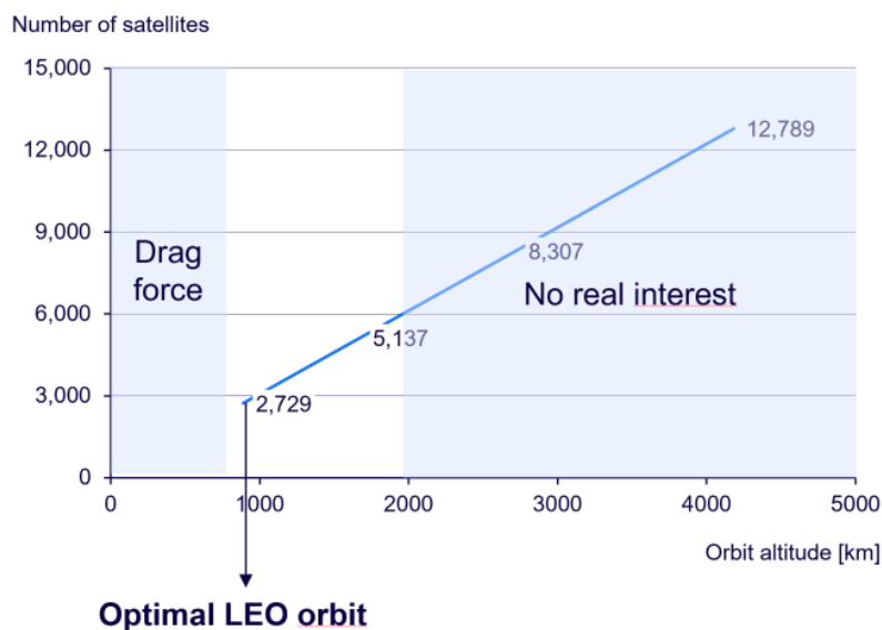
Figure 3 - Number of 1km diameter satellites for an orbit to reach 1000W/m 2 on Earth
